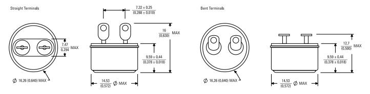
NOTE: Stud mount, surface and top mounting brackets are available. Dimensions listed are for reference only. Please contact Sensata for more detailed envelope drawings.
