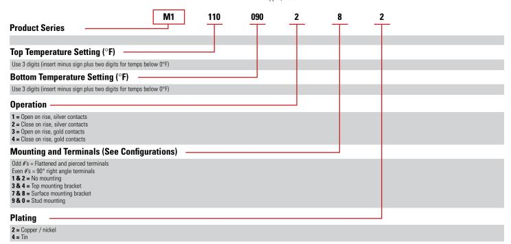
Configurations built to the standard tolerances and differentials are available as the M1 series and are described above.
